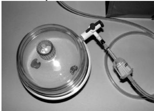
Figure 2 To use VAC-1D Desiccator Option (sold separately), plug Slip-Luer Filter into desiccator adapter tube, as shown. Refer to M1003 VAC-1D Operation Manual for more information
